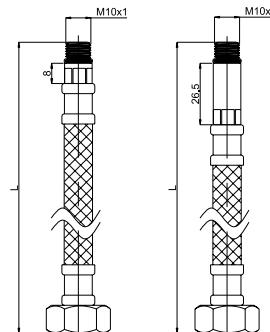
■ **M10xF1/2" stainless steel wire, EDPM rubber (short nozzle)**
